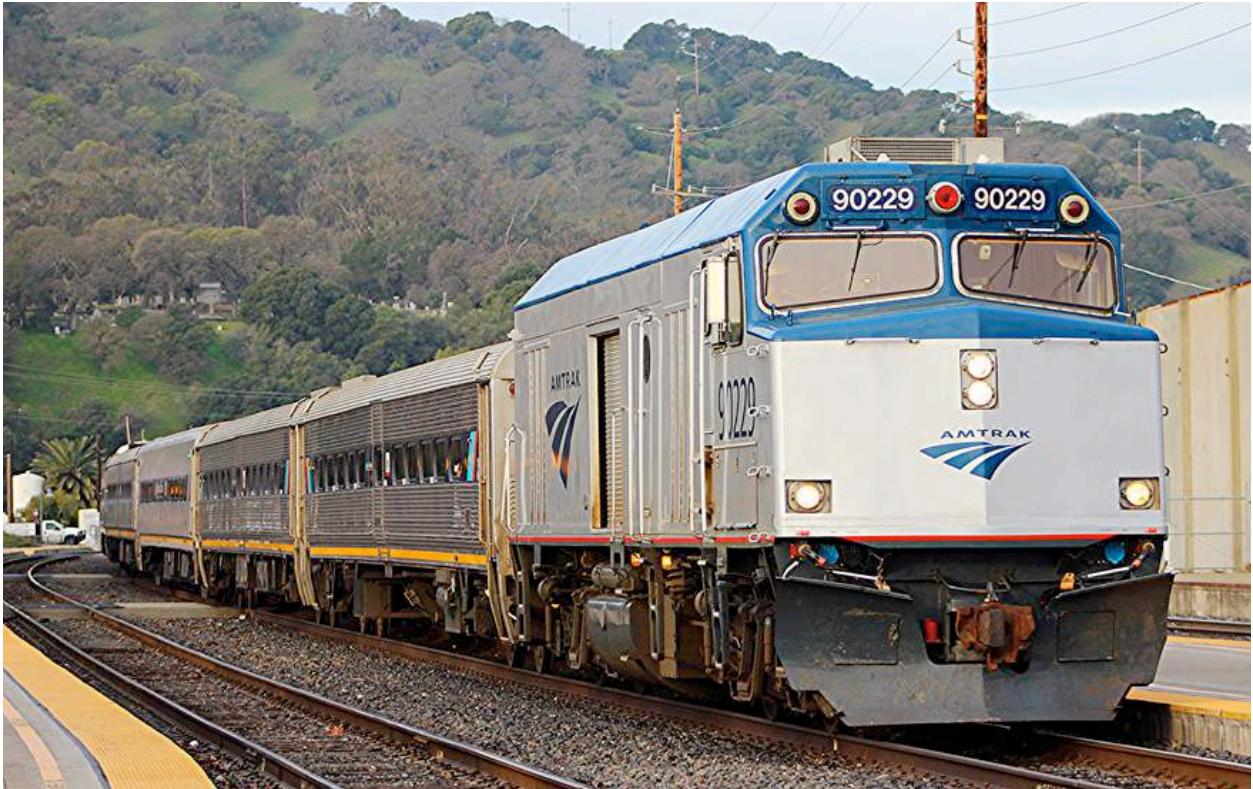
LOW-COST, MAKESHIFT PUSH-PULL OPERATION: In the absence of purpose-built HPR equipment, there are short-term methods for converting VIA’s uni-directional trainsets to push-pull operation. One is the Amtrak approach (above), which involves converting life-expired locomotives to un-powered cab cars. Another one that has been occasionally employed by VIA (below) simply uses locomotives on both ends of a trainset. Photos by Jamie West (above) and Ray Farand (below)
